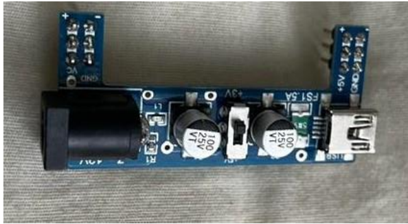
Figure 4: AMS1117 Power Module
